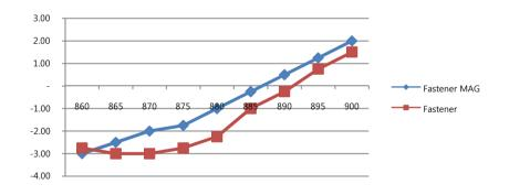
•FASTENER MAG reads up to 5.0 meters on metal, 20% shorter than FASTENER. Its read performance varies upon tag location, orientation, direction, RF environments, etc.
